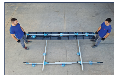
Traversi smontabili per lastre strette Dismantable cross bar for narrow slabs
